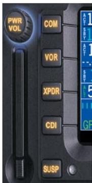
The **COM** key activates control of the Com radio. The Com radio window on the left side of the display will be outlined.
